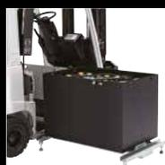
The optional battery roll-out feature allows easy replacement without a crane. Replacement time is significantly shorter and hoisting the battery unit is unnecessary.
